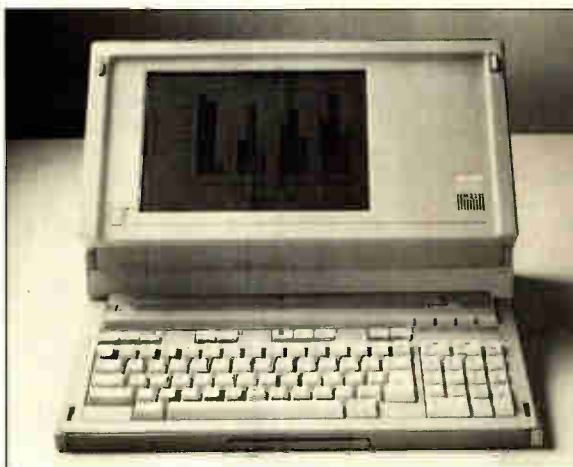
BACKLIT. Olivetti's 16-lb IBM PC-compatible computer has a backlit liquid-crystal display screen with six brightness levels.
