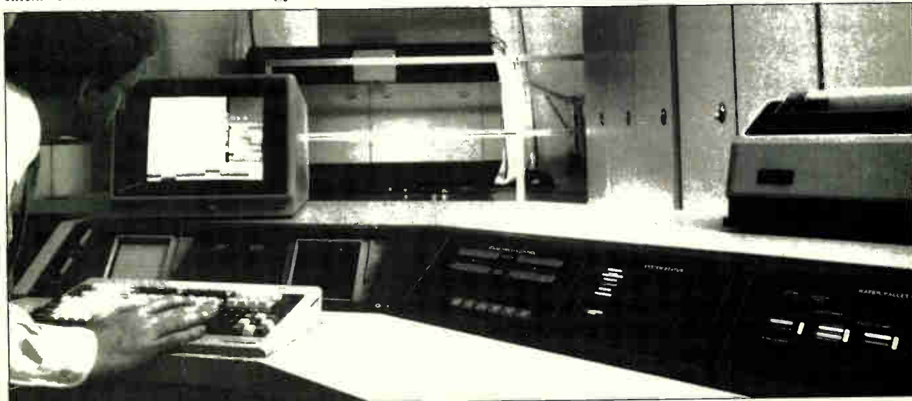
READY TO ROLL. Perkin-Elmer plans to ship this month the first high-throughput Aeble 150 electron-beam system for 0.5- \mu\text{m} work.
