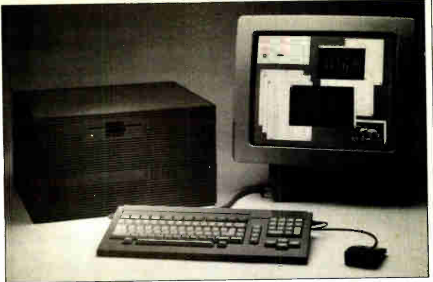
3. SMARTLY DRESSED. The flexible, expandable System 19 product family comes in a 5-in.-high plastic-sheathed case. As systems expand, modules neatly snap together.
