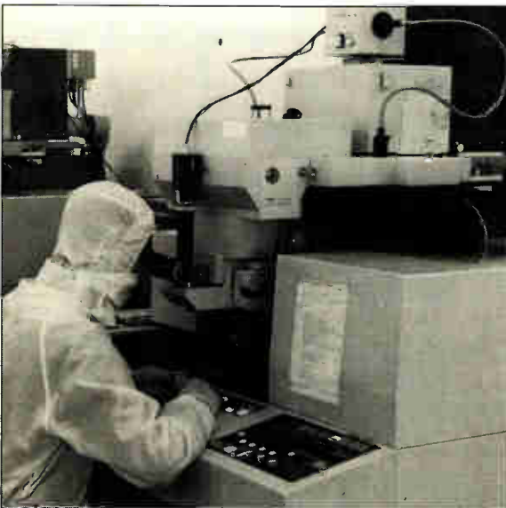
WHISTLE CLEAN. Critical fab operations, such as photolithography, are carried out in Mietec's class 10 clean room.
