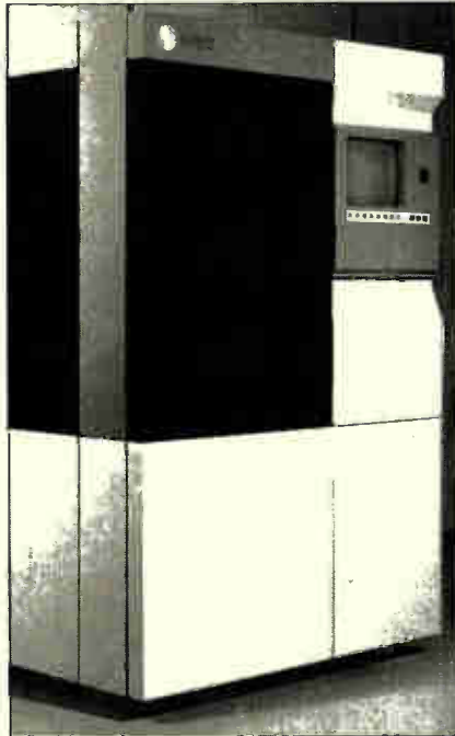
NO DAMAGE. The Aries etcher uses little pressure and does not undercut wafers.
