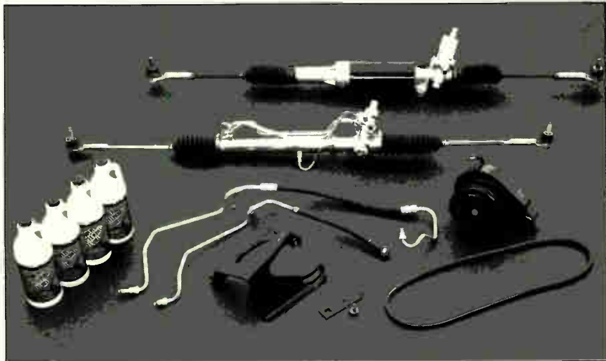
SIMPLER AND LIGHTER. TRW's electronic steering actuator (top) has only three major parts and weighs 28 lb. The hydraulic unit it supplants has 18 parts and weighs 35 lb.
