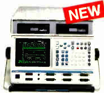
NEW K450. All high-speed channels: 10ns resolution across 48 channels at 100 MHz or 5ns across 24 channels at 200 MHz. 5ns glitch capture on all channels with no loss of memory. 4K memory depth. Unique Auto Save for saving failures in unattended mode.
