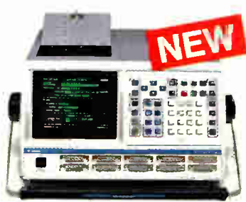
NEW K115. "The \mu P analyzer." Up to 72 channels for state/timing, 200 MHz on up to 8 channels. All key software/hardware integration tools, noise margin analysis, tolerance compare. Trace Control Multi-level "Help" Disassemblers for all popular \mu Ps, incl. 68020.
