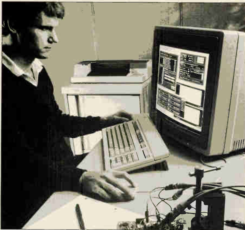
FOLLOWING THE PATH. HP's 3565S uses multiple-input/output frequency response so it can track what's going on in 62 instrumentation channels simultaneously.
