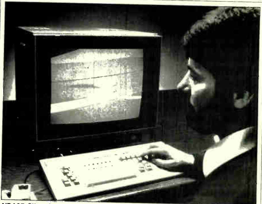
AIRACE. Silicon Graphics' new 3-d system does 86,000 transformations per second, suiting it for real-time graphics such as flight simulation and mechanical CAD.
