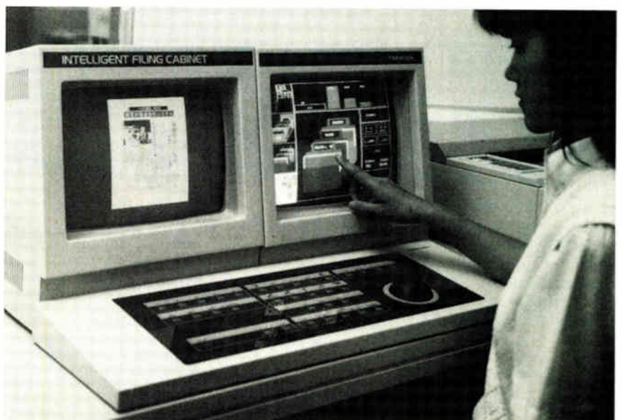
Graphics search. User presses touch-sensitive color CRT to access document from file cabinet displayed on screen. The document can be read on the adjacent monochrome screen.
