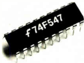
The 74F547 Decoder/Demultiplexer with Address Latches and Acknowledge.
