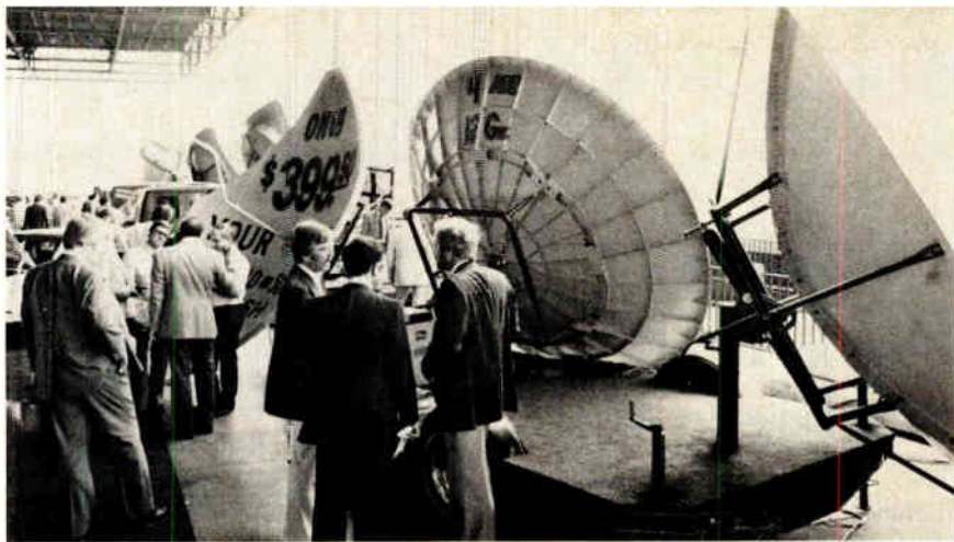
Backyard display. Some 13 exhibitors showed off their home-satellite earth station equipment at the Consumer Electronics Show earlier this month. Seen here are the 9- to 12-ft parabolic dishes that receive TV signals being relayed to earth by broadcast satellites.
