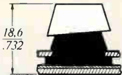
Actual size cutaway of low-profile actuator module
