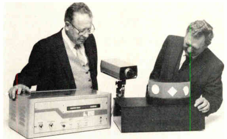
Robotic. William J. Heinecke, left, and Lawrence A. Murray of Electro Optical Integrated Controls eye the prototype of their Vuebot 301 robot controller. Shapes on the wheel indicate parts' shapes that can be identified using the CCD camera.
