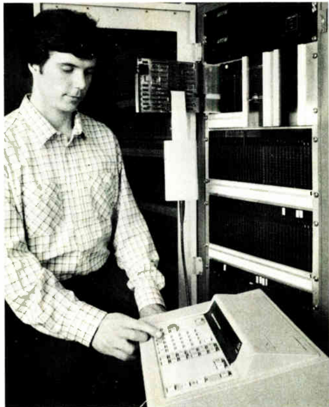
6. Smart service. John Fluke Manufacturing Co.'s 9010A is similar to IBM's maintenance device (Fig. 5), but lacks some of the latter's interfacing ability at present. It speeds service routine generation by learning board layouts and applying "canned" tests.
