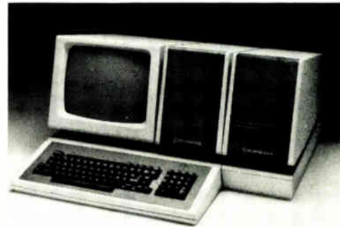
Starter. Model 680/10 single-user computer from CIE Systems starts at $8,700 with 128-K bytes of main memory.
