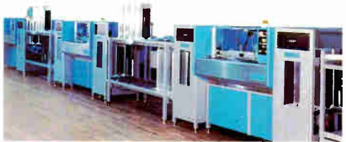
Pass-Thru modules provide buffer storage of circuit board magazines to integrate a line of automatic assembly machines with different insertion rates.
