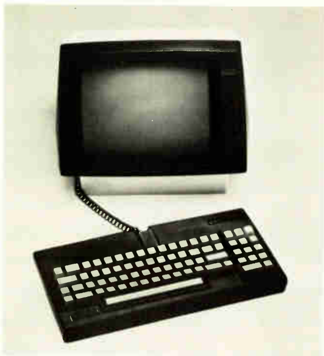
Designed for people. These two products, the Datapoint 8600 processor and the ADDS Viewpoint terminal, are designed with ergonomic features like low-profile detachable keyboards and tilting, swiveling screens.
