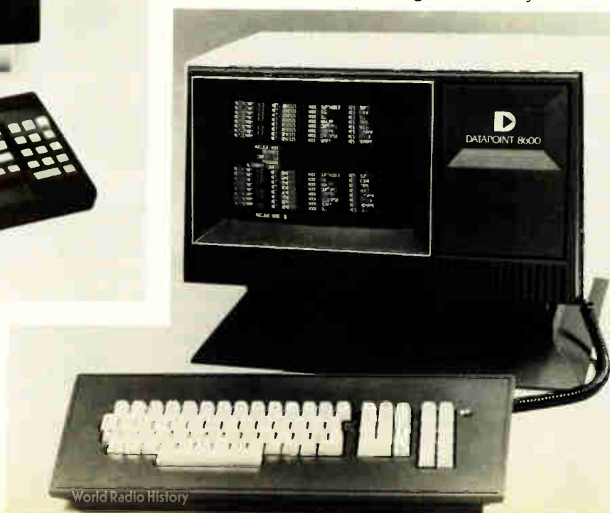
Designed for people. These two products, the Datapoint 8600 processor and the ADDS Viewpoint terminal, are designed with ergonomic features like low-profile detachable keyboards and tilting, swiveling screens.
