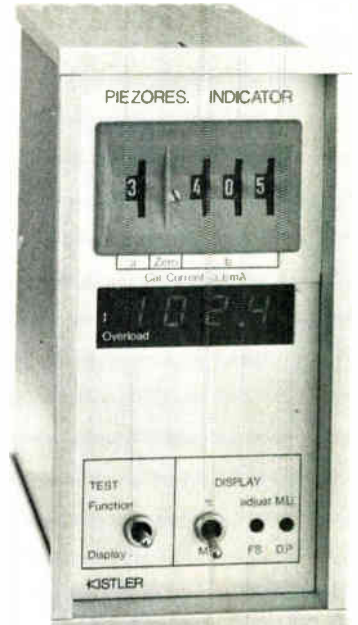
Type 4621 digital indicator, for piezoresistive transducers, has a 3 1/2-digit display and a selectable indication in units or percentages of the measuring range. It has an output of \pm 10 V at 5 mA with an impedance of 10 \Omega . Kistler AG, CH-8408, Winterthur, Switzerland [455]
