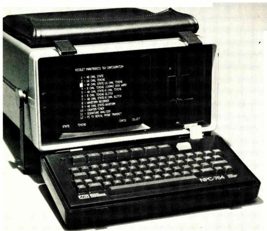
New breed. Nicolet Paratronics' NPC-764 logic-analysis system is one of the new breed of instruments whose computing power can be used by a knowledgeable operator.
