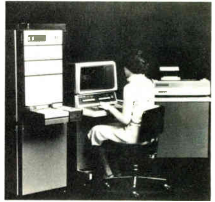
The T357 discrete semiconductor test system probes wafers, conducts final and quality-assurance tests, and in general evaluates a wide range of devices. It has a 64-K-byte memory, dual 3M tape drives, and software. Teradyne Ltd., Clive House, Queens Road, Weybridge, Surrey KT 13 9XB, England [442]
