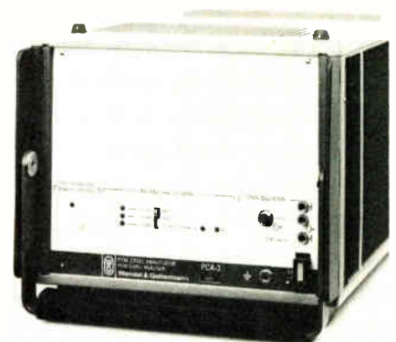
The PCA-3 pulse-code-modulated codec analyzer is a reference decoder for single-channel PCM signals. Testing follows recommendations of the International Consultative Committee for Telegraphy and Telephony. Wandel & Goltermann, P. O. Box 45, D-7412 Eningen, West Germany [444]
