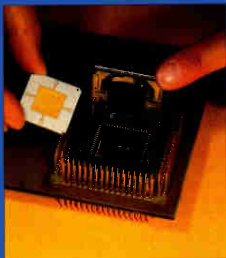
Solder type or surface compression type sockets accommodate all families of leadless Type A chip carriers of 68 terminals on .050" centers.
