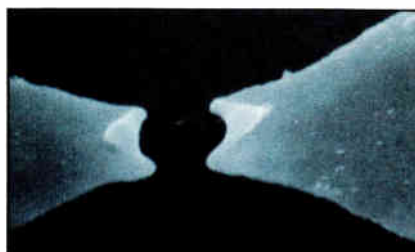
SCANNING ELECTRON MICROPHOTOGRAPH OF NATIONAL'S TITANIUM-TUNGSTEN FUSE IN THE OPEN STATE.
