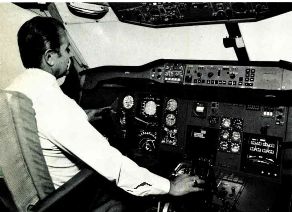
Full color and computerized. The A-310 Airbus will have an instrument panel with six CRTs: two in front of the pilot, two in front of the copilot (not shown), and two between them.
