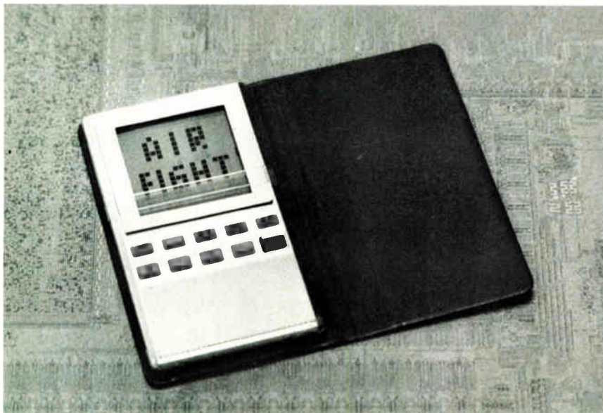
11. Fun calculator. Making possible this vest-pocket-sized video game is LCD technology and a 4-bit microprocessor soon to emerge from Sharp. Of the C-MOS chip's 60 pins, 40 drive the display directly. The toy is sitting on part of the IC's die photo.
