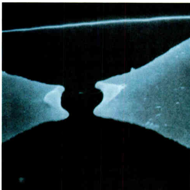
SCANNING ELECTRON MICROPHOTOGRAPHS OF NATIONAL'S TITANIUM-TUNGSTEN FUSES IN THE CLOSED AND OPEN STATE.
