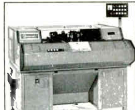
Model 4611 Hybrid Microelectronic Assembly Machine. Automatically places chip capacitors, integrated circuits and other microelectronic devices as small as 030" on substrates at cycle rates up to 3,600/hr
