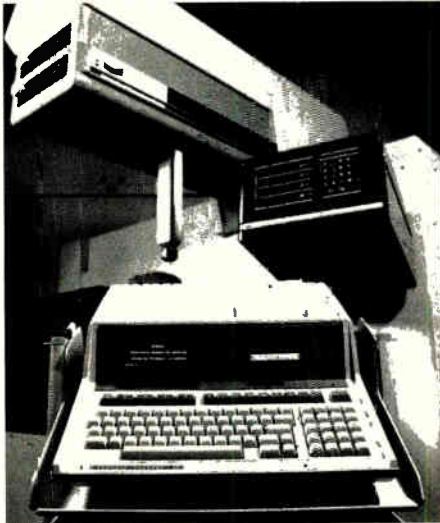
Bendix uses the HP-85 personal computer as the brains behind its coordinating measuring machines.
