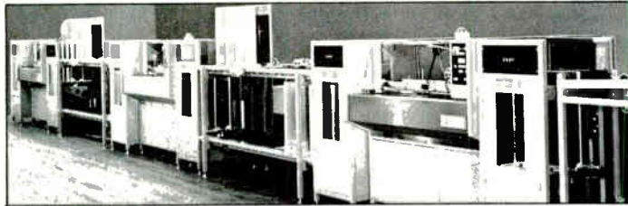
Pass-Through™ Automatic Board Handling System eliminates manual board feeding and removal. System accepts boards in slack or magazine input, moves them through the machine and accumulates inserted boards in a magazine loader for automatic movement to the next machine
