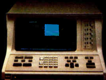
Hewlett-Packard 1610B A sophisticated data-domain-only logic analyzer
