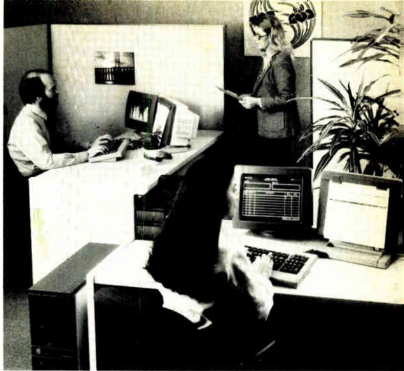
7. A boon in the office. The complete personal minicomputer for office use from Convergent Technologies is a three-piece desktop arrangement of keyboard, screen, and computer with lectern face. Disk drives are in floor-standing cabinets that fit neatly beside a desk.
