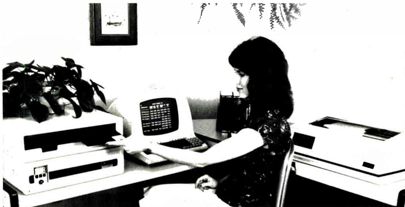
1. Network station. A local-network work station in the Z-Net system is truly a desktop installation. The MCZ 2/50 user's station shown has a display terminal and printer, both controlled by a Z80 microprocessor. More than one of these peripheral devices can be used if desired.
