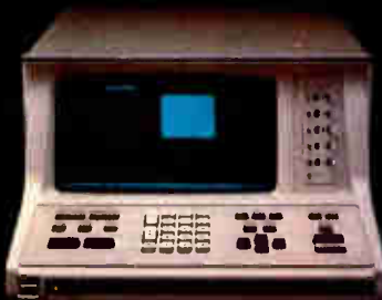
Hewlett-Packard 1610B A sophisticated data-domain-only logic analyzer
