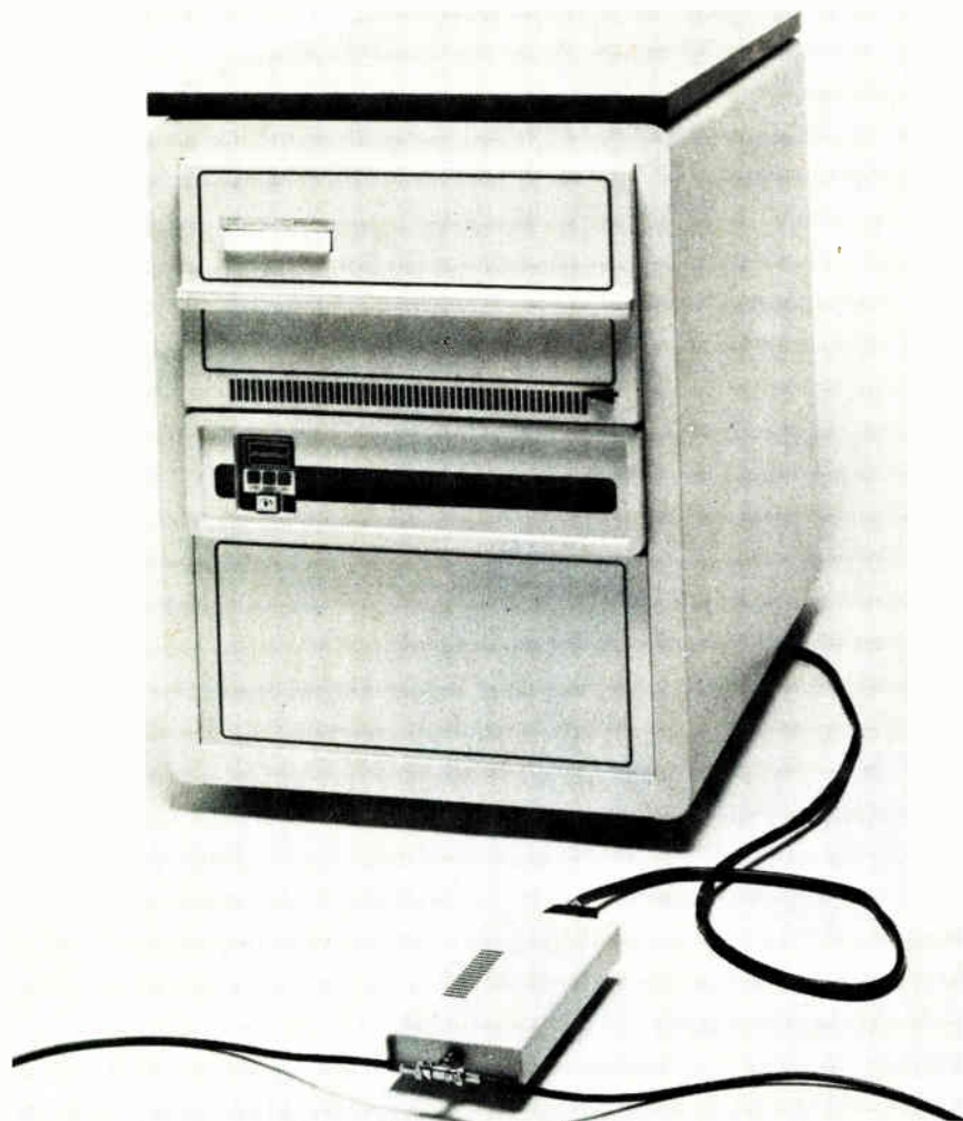
2. Many stations. Z-Net links as many as 255 of the various versions of the MCZ-2 series microcomputer systems with up to 7,000 feet of coaxial cable. The Z80A-based SDS 2/01 disk-drive unit shown lets data files on the system be shared without a central controller.
