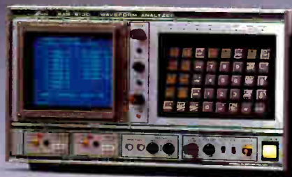
GP-18 Waveform Analyzer SAS-8130 (sampling: up to 12.4 GHz)
