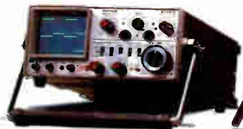
Mini Oscilloscopes (field service use: up to 50 MHz) photo: SS-3510)
