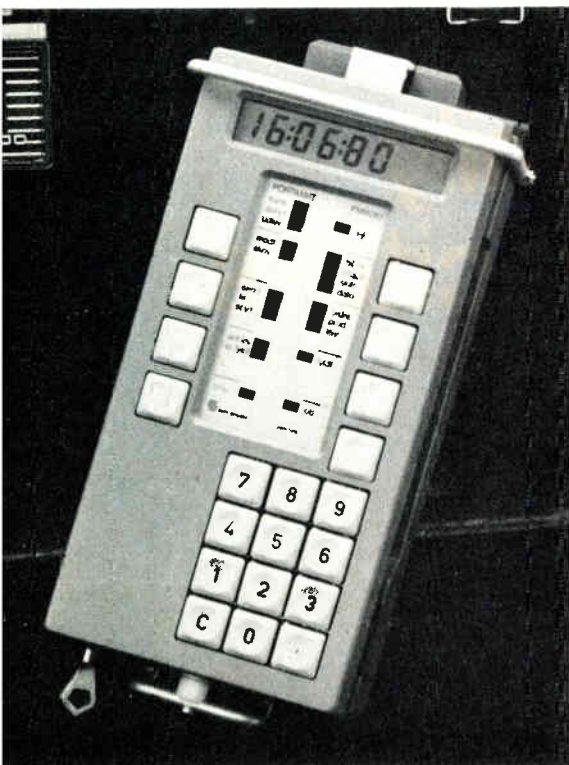
Automatic billing. Hand-held computer in holder in truck cab enables printer (not shown) to produce on-the-spot invoices from delivery data entered by driver.
