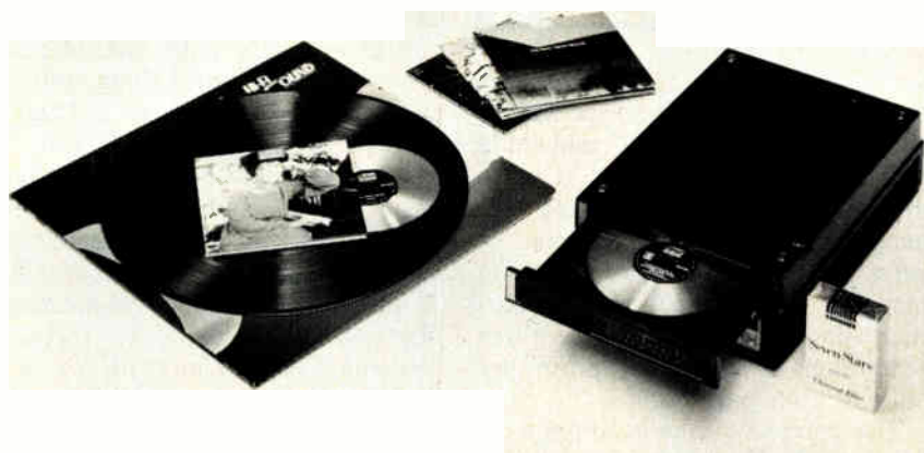
Future player. This prototype digital audio disk player was shown by Sony at the Tokyo audio show last October. Compatible with the Philips system, it is not a product yet.
