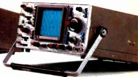
Oscilloscope SS-5421 (R & D use: 350 MHz)
