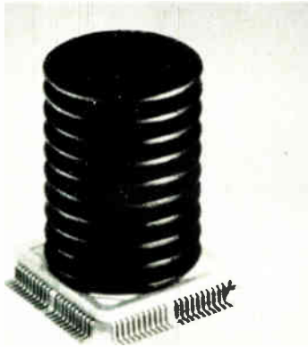
Air-cooled. Amdahl continues with air cooling in its new computers, now with 10-tiered towers on both the CPU chips (left) and on the four-chip RAM clusters.
