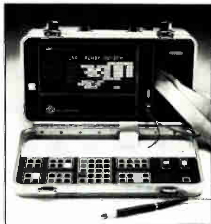
The MicroSystem Analyzer. Low cost board and system test for \mu P-based systems. Right down to the node level.
