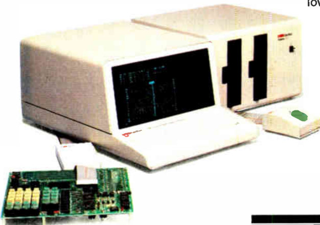
GenRad 2300 Series Stand-Alone Universal Development System. Supported processors: 8080, 8085, Z-80, 6800, 6802, 1802; the 8086 and 6809 are supported with the GenRad 2302 Slave Emulator.
