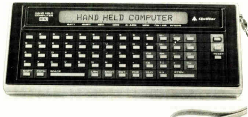
Handy data. This is the central processor for Panasonic's hand-held computer. Peripherals are packed in an attaché case. ROM capacity is about 40,000 words, RAM is 73 kilobytes.
