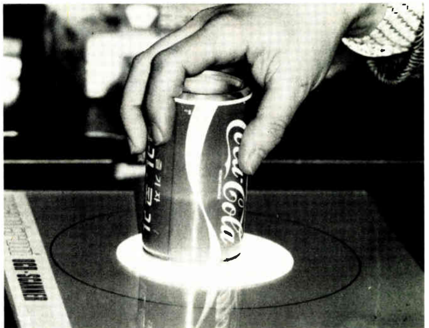
Quick study. TV-camera-like scanner uses 8-bit microcomputer to read 22-character label in less than a second. The goal is to topple bar-code-based systems.
