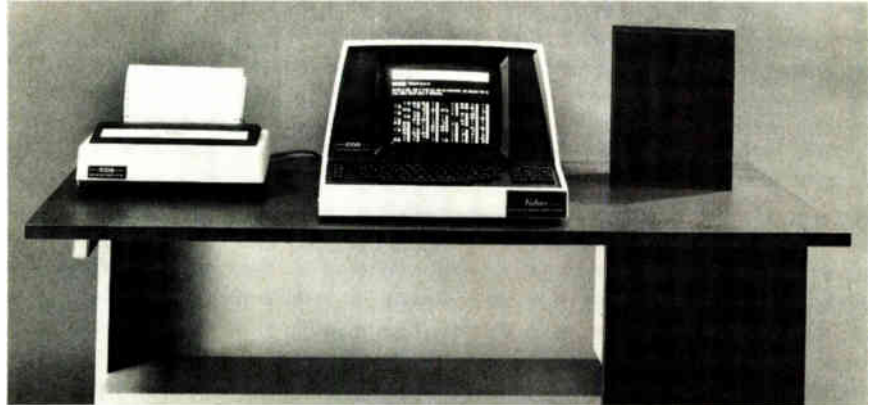
Speak up. Votrax's 6502-based development system converts typed words and phrases directly into spoken ones. Its algorithm simulates the rules for pronunciation.
