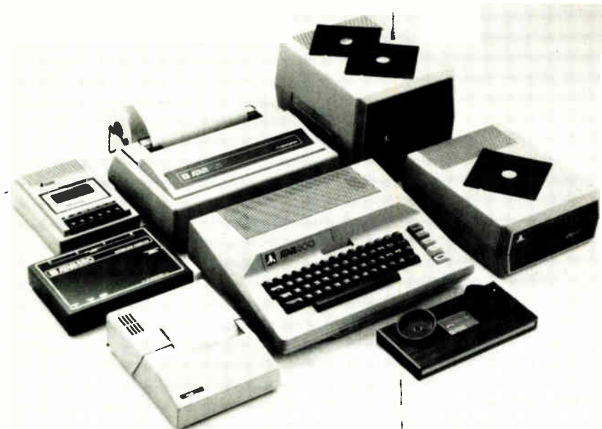
Shown off. Atari's line includes, clockwise from lower right, modem, microcomputer, thermal printer, interface module, program recorder, impact printer, dual disk drive, disk drive.
