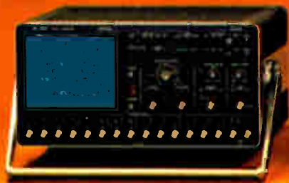
PM3500 100MHz 16 Channel Logic Analyzer
