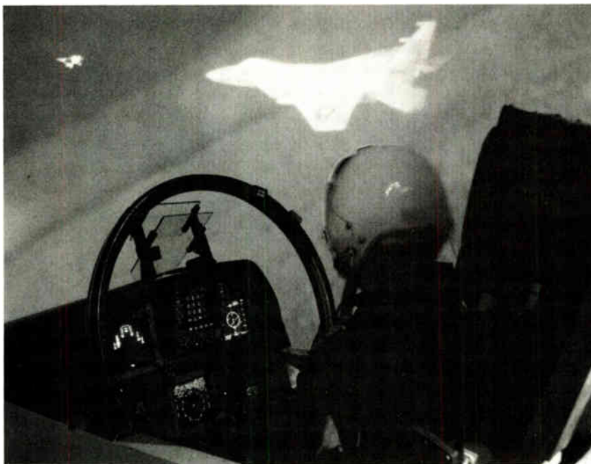
Fledgling. Pilot trainee in a Manned Air Combat Simulator from McDonnell Douglas practices formation flying without leaving ground. Image is on a 40-ft-diameter projection screen.
