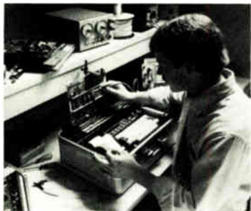
GenRad's 2225 is the first functional field service tester with automatic guided-probe fault isolation.
