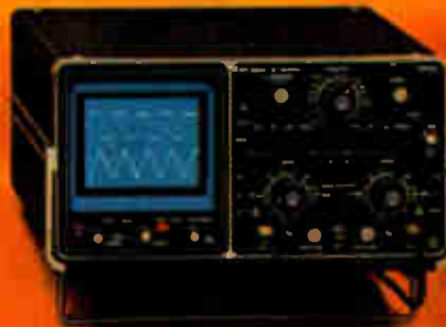
PM3234 10MHz Dual Beam Storage Scope
