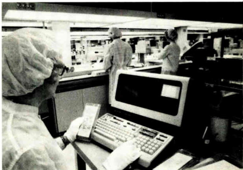
4. Wafer logging. An operator is pictured logging wafer and material movement into a cathode-ray-tube terminal. This information is stored in the factory management computer and is used to monitor the flow of wafer lots through each station in an MOS process.
