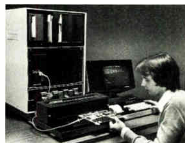
For high-volume service depots, GenRad offers the 2225 compatible Omnicomp Logic Test System.
