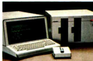
GenRad's Futuredata microprocessor development system is capable of programming and emulating—at full speed—all the popular microprocessors.
