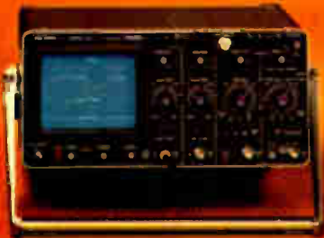
PM3262 100MHz Dual Trace Universal Scope
