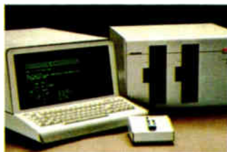
GenRad's Futuredata microprocessor development system is capable of programming and emulating—at full speed—all the popular microprocessors.
