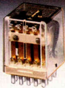
NEW 5-Pole KH Relay. 5 form C version of popular KH relay is only slightly larger than present 4 form C model. Rated 3 amps at 30V DC, resistive, or 120V AC. 100,000 operations minimum. Available with plastic dust cover or hermetically sealed in a steel case.
