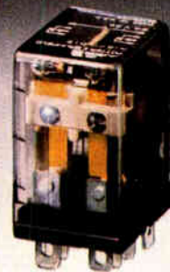
NEW K10 General Purpose Relay. Space-saving relay has contacts rated 10 amps at 28V DC or 120V AC, resistive, 100,000 operations minimum. Contact arrangements to 2 form C. Ruggedly constructed for use in alarm systems, control assemblies and other applications requiring 10 amp switching in a limited space.
