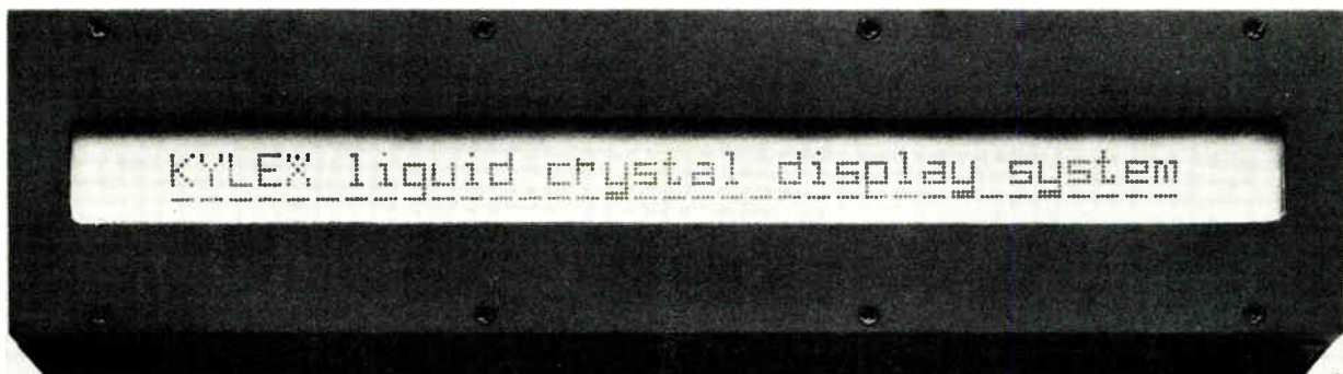
1. Forty characters. Photolithographic techniques, instead of the usual screen printing, allow closer spacing of the dots in the Kylex LX140 liquid-crystal display. An advance in LC materials made a new level of multiplexing complexity possible; internal circuitry eases interfacing.
