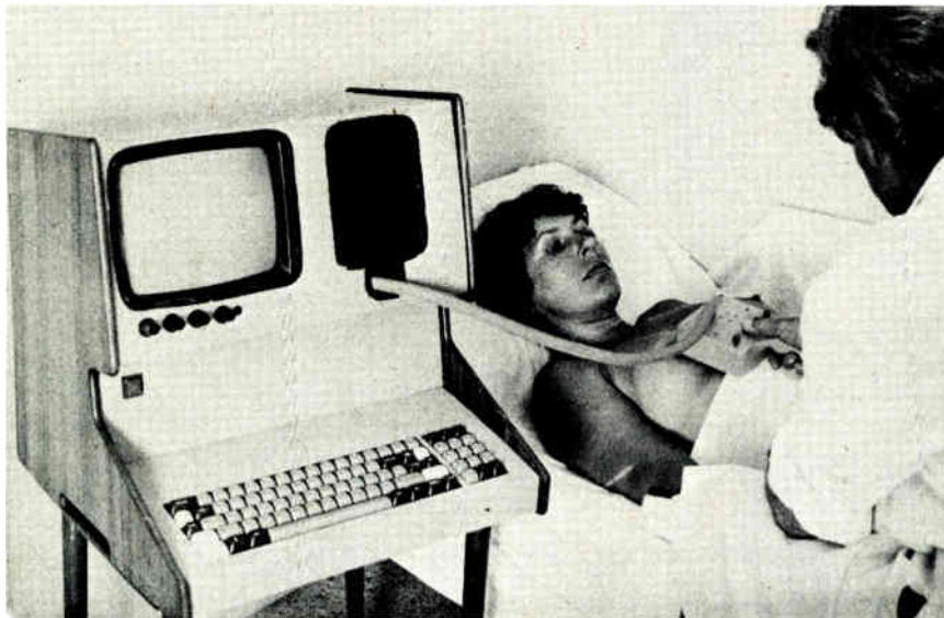
Safe, simple. Mammo-scaner from Israel's Weizmann Institute of Science detects breast tumors by measuring dielectric properties. Hand-held probe contains 64 sensors.
