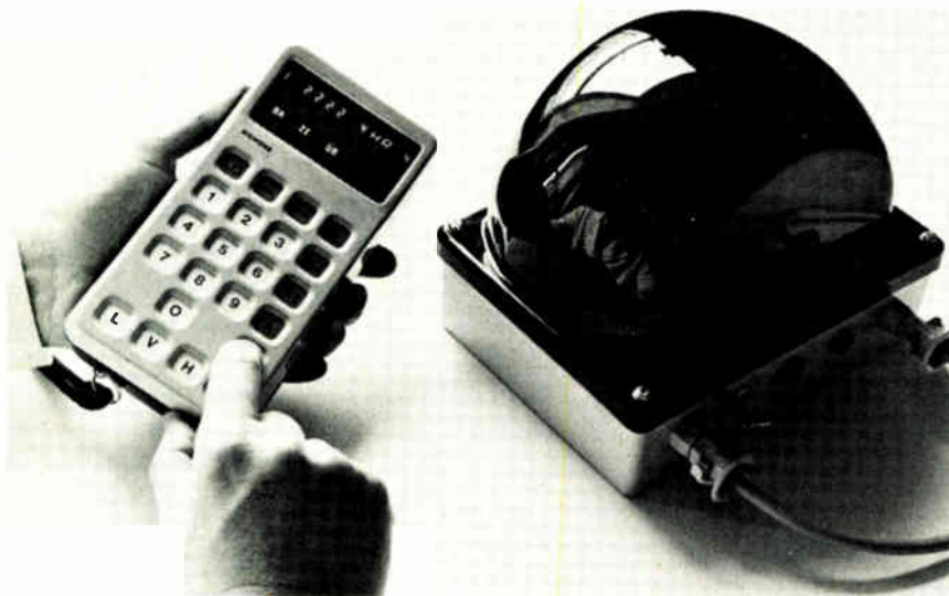
Beaming in. Siemens' data-input system links a portable, calculatorlike terminal (left) via IR beams to a "data collector" (right), which is connected to a computer by wires.
