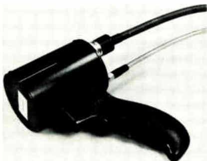
Double duty. Microwave system uses one assembly for detecting and treating cancer. Small white rectangle is detector antenna; big one around it is treatment antenna.
