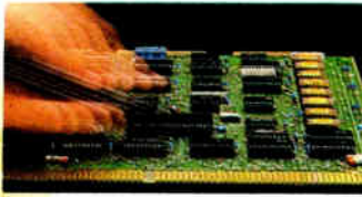
GenRad's in-circuit test systems employ a simple SCRATCHPROBING™ technique to quickly pinpoint faults—cutting labor costs up to $50 a board.
