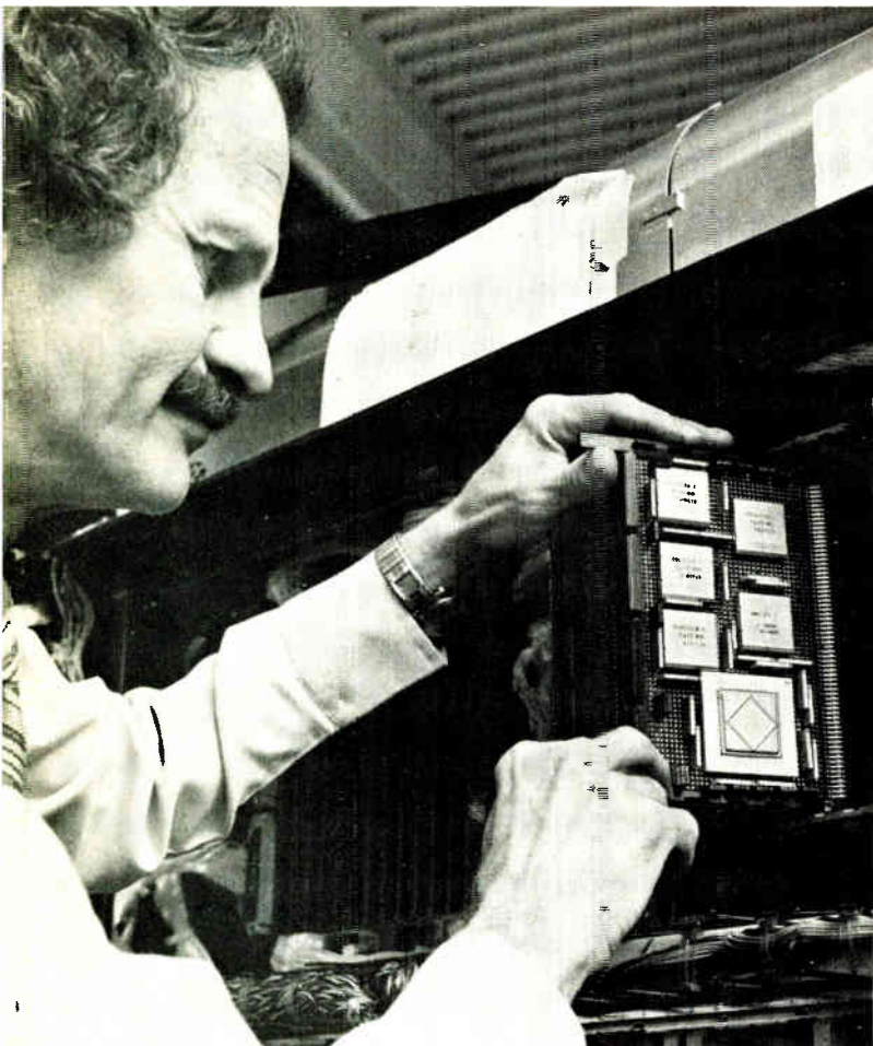
Future directions. IBM Corp. views master-slice chips containing arrays of 704 gates as the best way for it to employ large-scale integrated circuits in future computers. Shown here are the new logic elements being installed in the new 4300 computers.
