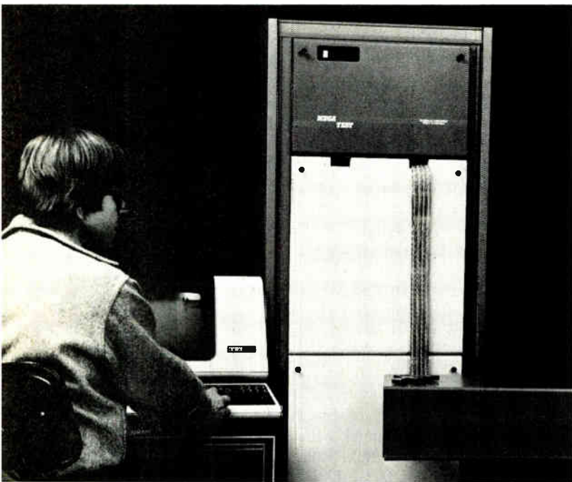
Magnetic provinces. The magnetic-bubble memory testing world was divided into three parts with the introduction of commercial test systems from Fairchild Camera and Instruments' Xicom division, Megatest (whose system is shown above), and Watkins-Johnson.
