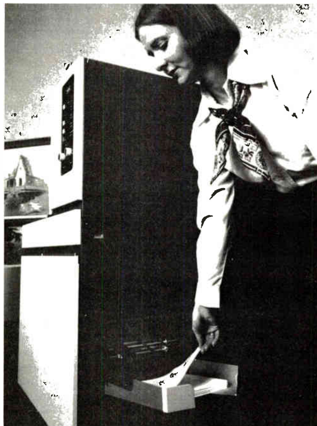
Quality copy. By combining a xerographic copier with a cathode-ray-tube display, Wang Laboratories succeeded in producing a nonimpact printer that can produce output of correspondence quality at rates of up to 18 pages a minute.
