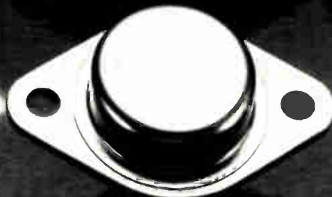
Family: 2N6284 (N-P-N), 2N6287 (P-N-P). Current range, amps: 20. Voltage range, V_{CEO} (sus): 60-100.
