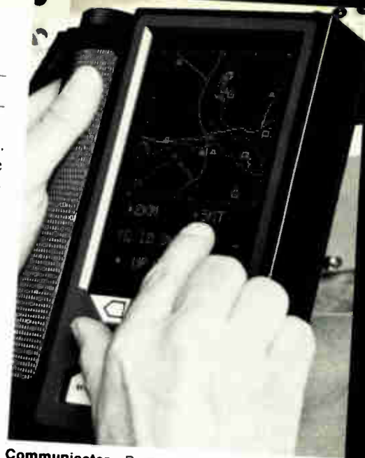
Communicator. Book-sized terminal displays alphanumeric and graphics on LEDs.
