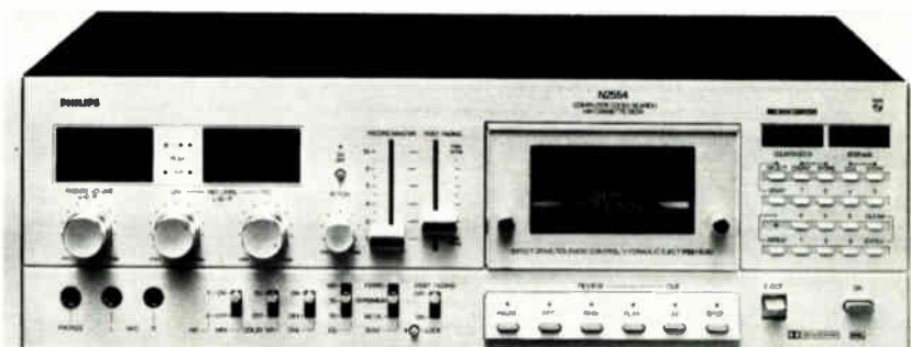
Smart deck. Philips' audio cassette unit can record inaudible code signals to mark the start of each taped selection; a special head reads the codes even during fast winding.
