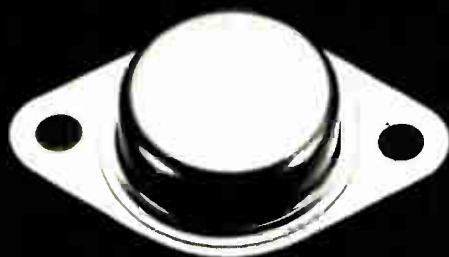
Family: RCA 8766. Current range, amps: 10. Voltage range, V_{CEO} (sus): 350-450.
