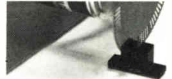
opto electronic switch with self-contained Schmitt conditioning circuitry
