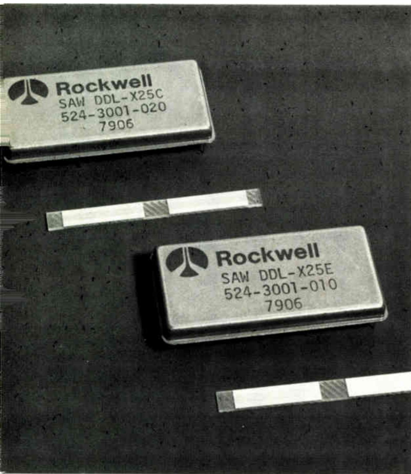
7. A pair. A typical 100-MHz expansion and compression filter pair may readily be implemented in dual in-line packages. Plastic or TO-8 cans are possible alternatives, depending on the application, while machined parts may be necessary for some custom designs.
