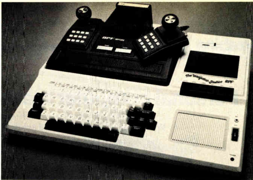
Think about it. The Imagination Machine is from APF Electronics Inc. of New York. This home computer features 10 kilobytes of ROM, 9 kilobytes of RAM, and eight-color graphics.
