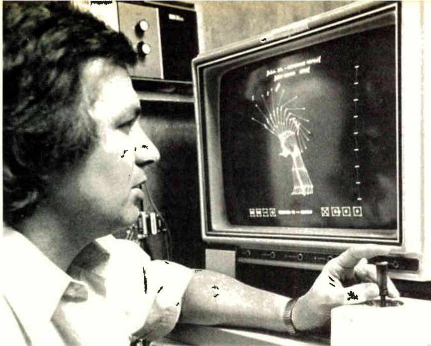
Stick man. Gideon Ariel adjusts stick-like figure on CRT display, which he uses to judge how slight modifications in what an athlete does may affect overall performance.
