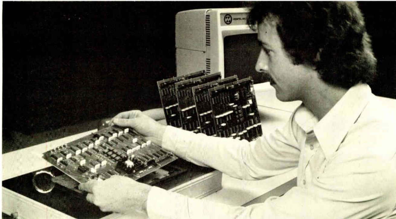
2. Coping with LSI. The Zehntel TS800 employs low-impedance drive for device isolation, coherent stimuli to excite device inputs, and signature analysis to detect faulty LSI devices. The system is also capable of conventional analog in-circuit testing.
