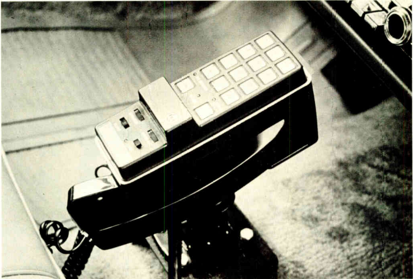
5. Who's calling? Except for some extra digits that are necessary because the customer is calling from a mobile unit, the car telephone works much the same way as an office phone. Incoming calls are perceived as beeps on a built-in loudspeaker.
