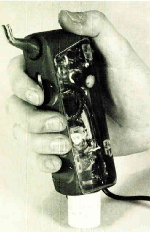
Hand-held cancer killer. Interior of prototype rf hyperthermia applicator shows miniature 2-megahertz oscillator and temperature-control circuitry. Unit can help manage up to 90% of cattle cancer-eye cases.
