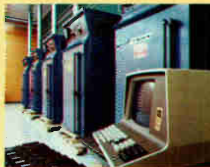
For high reliability all Cromemco memory cards are burned in at the factory in these temperature-controlled ovens.
