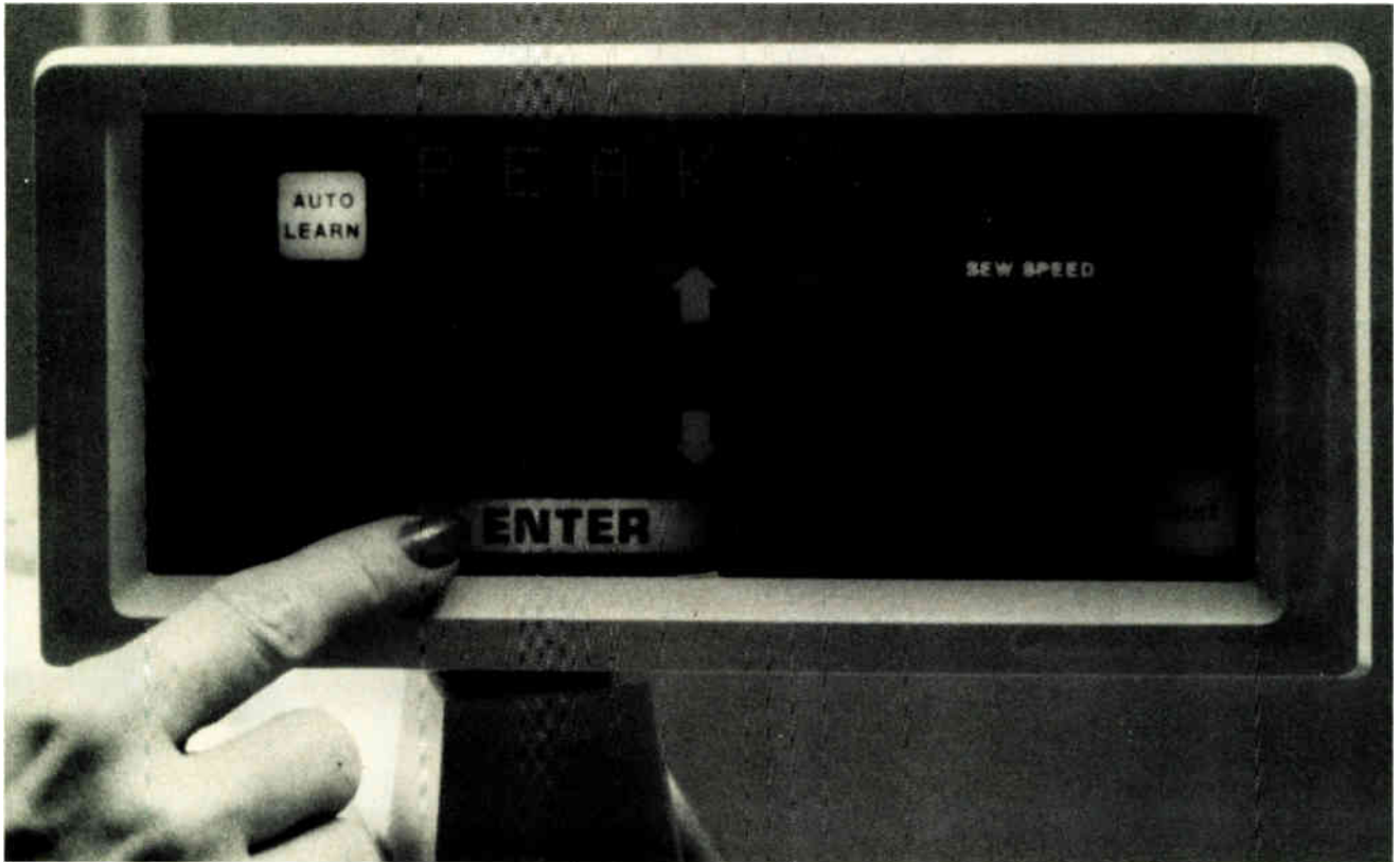
2. A stitch in time. The industrial model uses a microprocessor to speed repetitious work. In the learning mode, the machine records the stitch sequence and the speed of the operator. When switched to auto-sew, it repeats the sequence as the operator moves the material.
