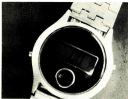
Time beats on. Sensor to measure heart rate is on the face of digital watch. The user puts an index finger over the sensor to get a reading displayed every 5 seconds.
