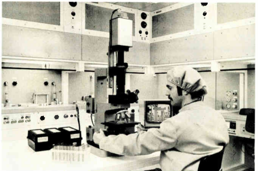
Clean job. Inspector checks circuit in super-clean environment of mask-making center at ITT Semiconductors' new research and development facility in Freiburg, West Germany.
