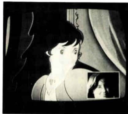
TV extra. Inset picture in Hitachi TV system has less resolution than does the main picture but is adequate for its size.
