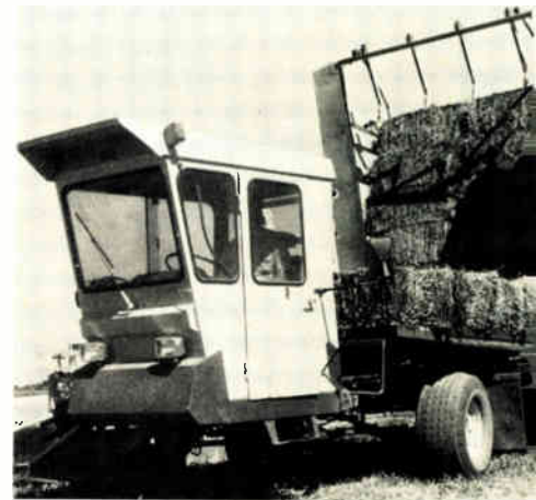
Baler. Loading operation in Sperry New Holland automatic bale wagon is sequenced by an on-board C-MOS digital control unit.
