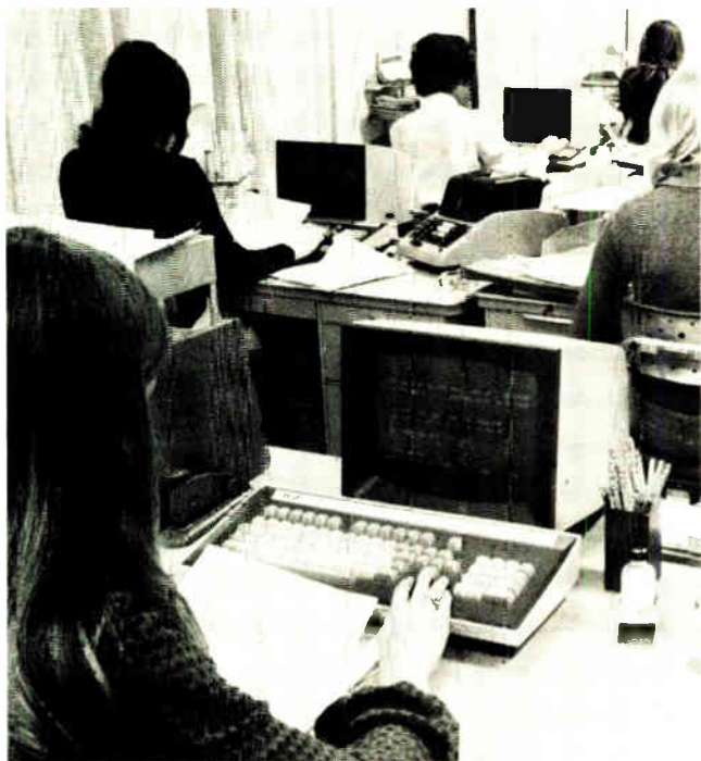
8. Under the umbrella. Some vendors without network architectures have chosen instead to operate under the umbrella of IBM's SNA. Four-Phase Systems' clustered terminal units, for example, do stand-alone data processing yet link into a host IBM mainframe.
