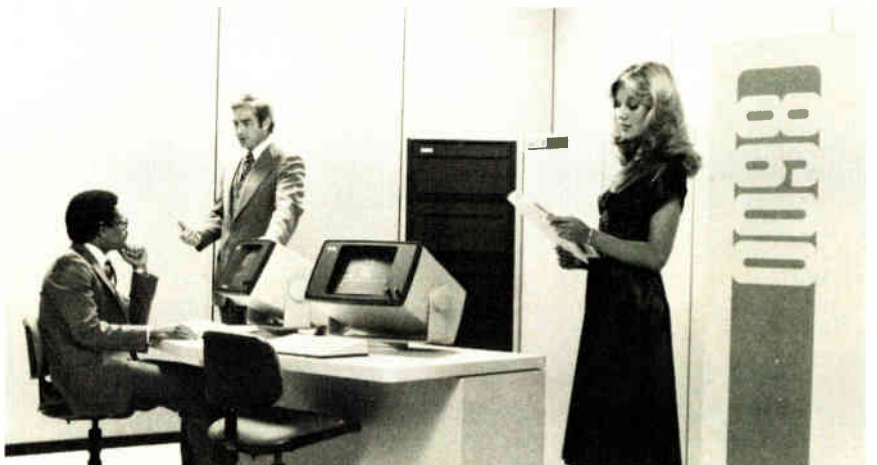
Powerful. Top-of-the-line V-8600 central processor, most powerful yet introduced by NCR, uses 64-kilobit random-access memory chips and fast emitter-coupled-logic 100K circuitry.
