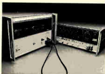
5200A AC calibrator and 5205A power amplifier.
