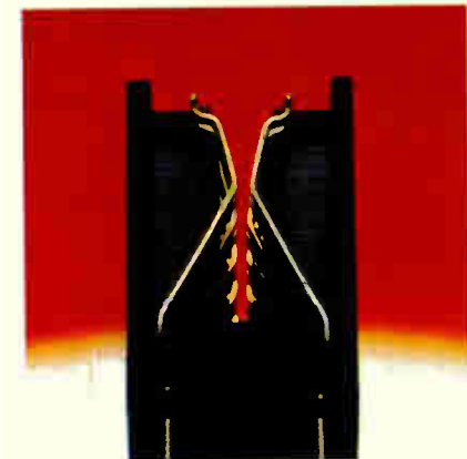
Cross Section of H4 Series Edgeboard Connector
