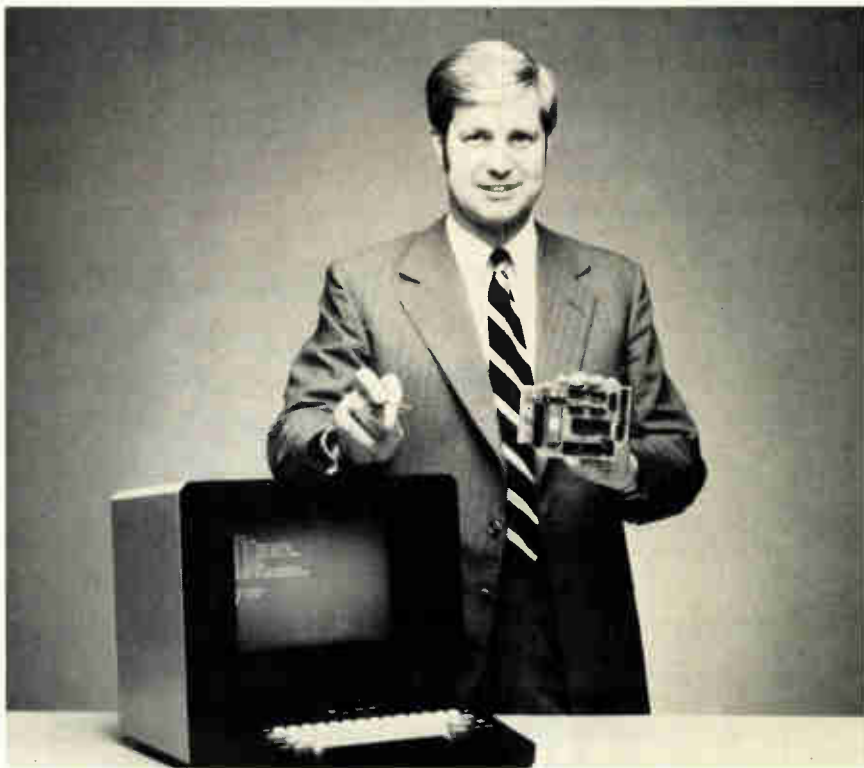
Terminal. Perkin-Elmer's David Ratcliffe leans on the Bantam terminal holding the key to its design—an LSI microprocessor-and-controller chip—and the components it replaces.
