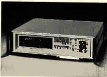
The 8502A \mu P-controlled DMM.
