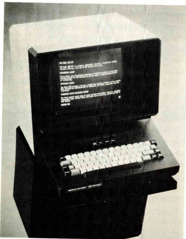
Changing display. Cathode-ray-tube-display manufacturers are taking advantage of chip technology to pack more intelligence into less space. Perkin-Elmer's Data Systems group combined a microprocessor and CRT controller on a single chip in its 550 terminal.
