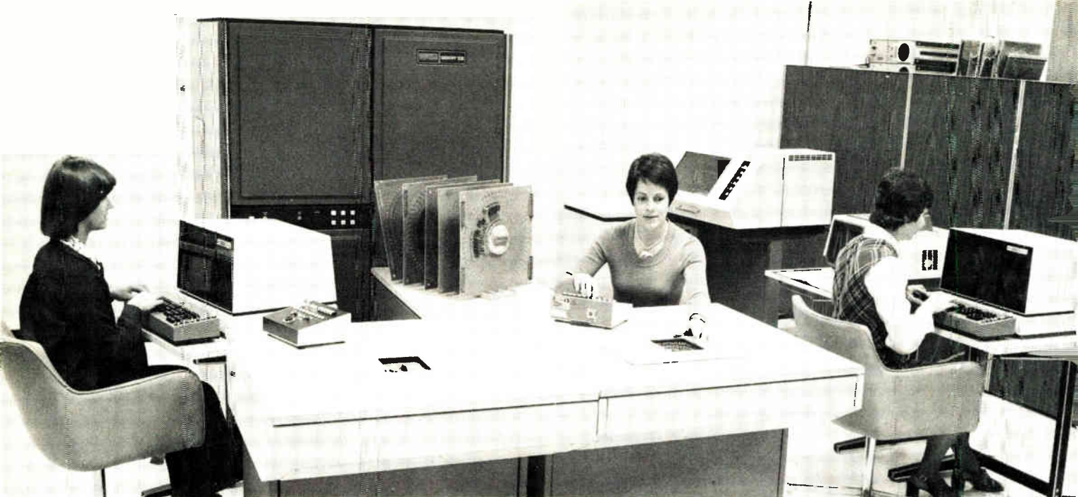
1. Sentry. The Sentry series of automatic testers from Fairchild Systems Technology includes computer control unit (background), programming stations (left and right), and multipin test heads (foreground). Shown is the latest in the series, the Sentry VIII.
