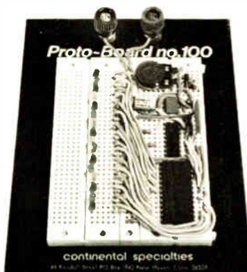
Proto-Board ® 100, 760 solderless tie-points. Kit, $19.95*
