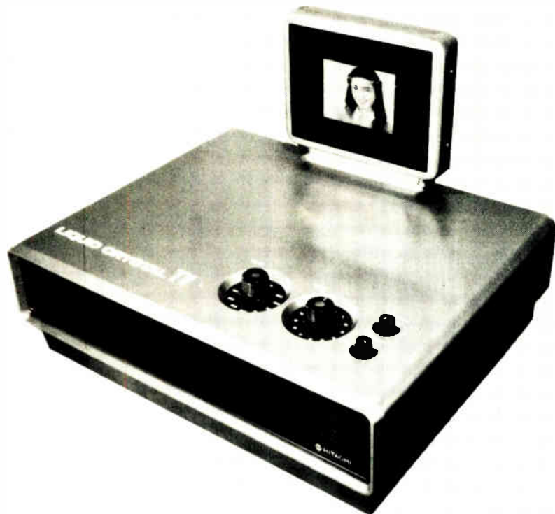
LCD. Display area of liquid-crystal TV screen from Hitachi is 120 mm wide, 90 mm high. It is 4(1) mm thick. Picture elements are selected by matrix-addressing technique.
