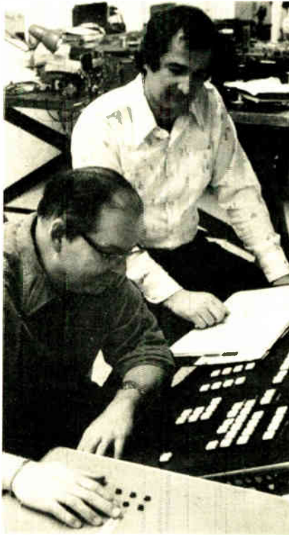
Alternative. Braille cells (white strip at bottom) spell out information normally provided on lighted push buttons and lamps.
