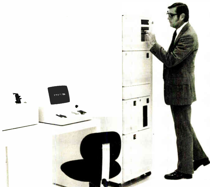
Complete series. IBM's Series/1 minicomputers include processor, fixed disk, and floppy disk in one 19-inch rack, plus a CRT display and serial printer as two separate units.
