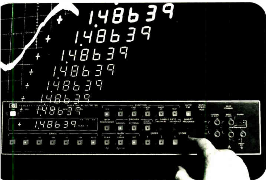
HP-IB New 5 1/2, 6 1/2-digit DVM checks its dc and ohms circuits for accuracy and then makes corrections. One microprocessor controls the Auto-cal process; the other is for computation of the math functions and remote programming via the HP-IB.
