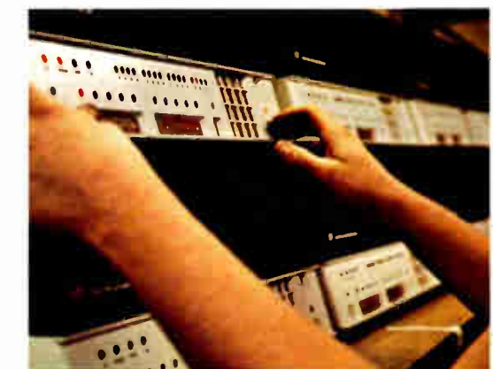
Computers awaiting shipment idle away the hours under test. Reliability benefits from the additional component aging.
