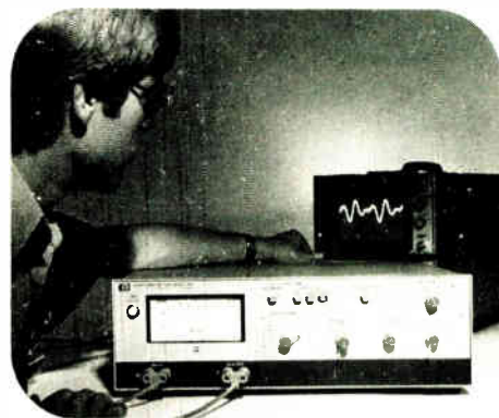
New distortion analyzer with distortion input sensitivity of 1 Vrms for 100% set level reference.
