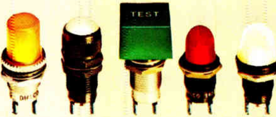
INCANDESCENT OR NEON SUB-MINIATURE INDICATORS —Meet or exceed MIL-L-3661. Mounts in 15/32", 1/2" or 17/32" clearance holes. Incandescent for 1.35-28V; neon has patented built-in current limiting resistor. Choice of cylindrical, faceted, convex, flat, square and round lens shapes, finishes, legends. Stocked by local distributors.
