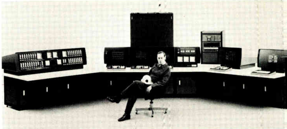
New look. Honeywell's new TDC 2000 process-control system connects microprocessor-based controllers and stand-alone CRT terminals to central computers via coaxial cable.
