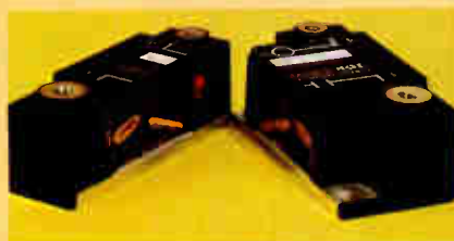
Cutaway photo shows complete encapsulation of components.
