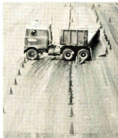
No skidding. Electronic braking systems prevent the brake locking that can lead to jackknifing and other dangerous skids. But some systems are proving faulty.
