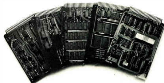
Five card 8080 microcomputer system. Includes microprocessor, 256-word instruction PROM with 2048-word capacity, and 1023-word program or data RAM with 4096-word capacity.
