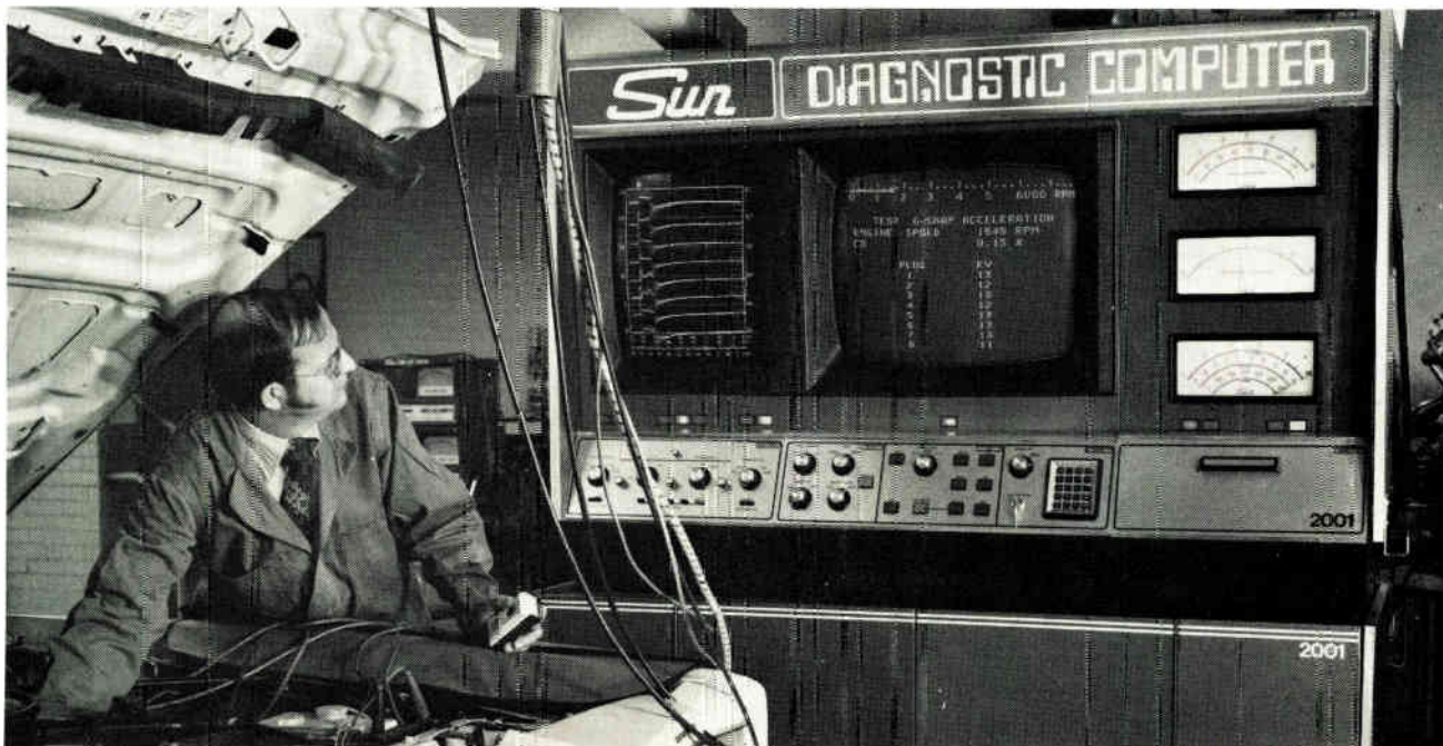
From the Sun. Model 2001 Diagnostic Computer from Sun Electric will sell for $13,950. It steps mechanic through test procedure.
