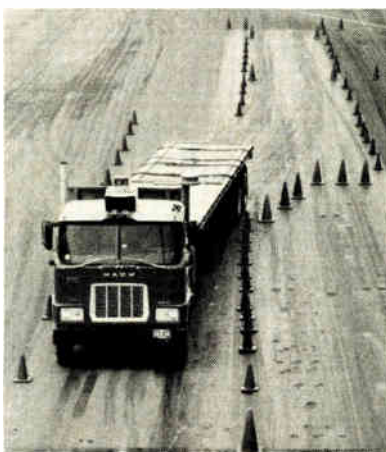
No skidding. Electronic braking systems prevent the brake locking that can lead to jackknifing and other dangerous skids. But some systems are proving faulty.
