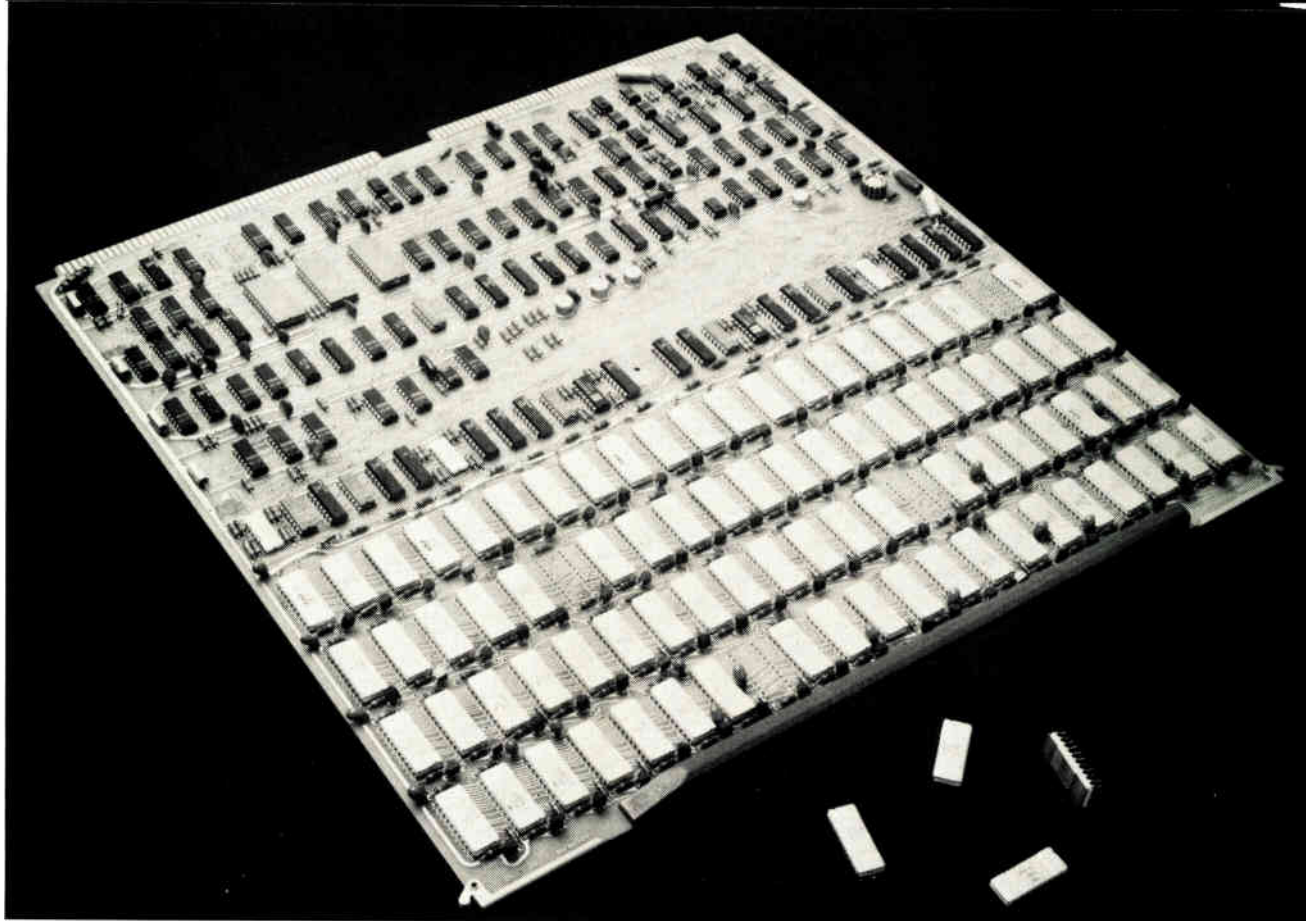
4. Memory board. The Eclipse semiconductor memory uses 2-kilobit chips and, with the error correction techniques, the memories have been operated with as many as four chips unplugged, simulating complete failures. Each memory module holds 8,192 words.
