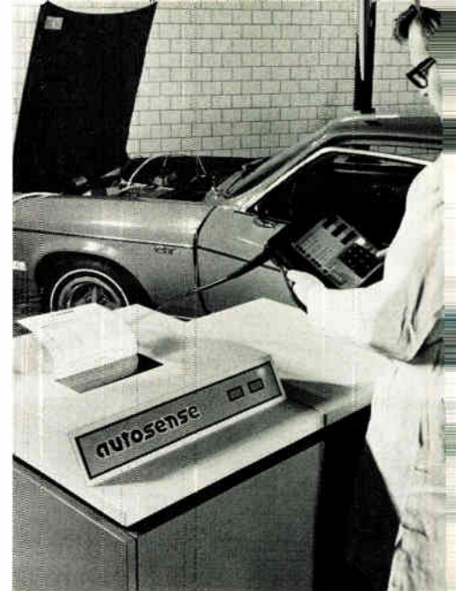
Autosense. That's what Hamilton calls its new auto-diagnostic system, built around a 16-bit minicomputer with a 4,000-word memory. It costs up to $11,900.
