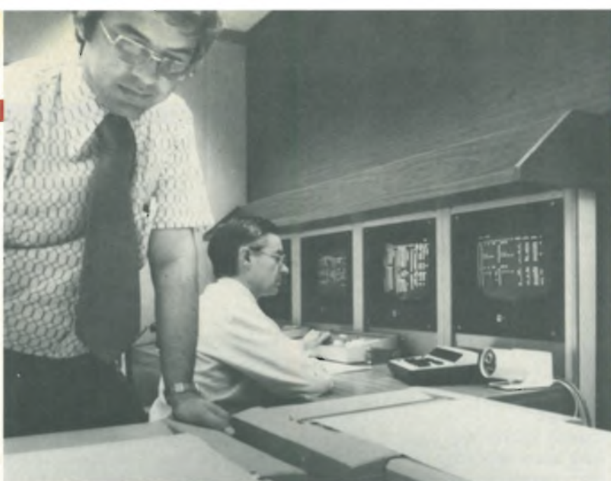
Condensed information. CRT displays, such as this console designed by TRW Controls, monitor petroleum pipelines.
