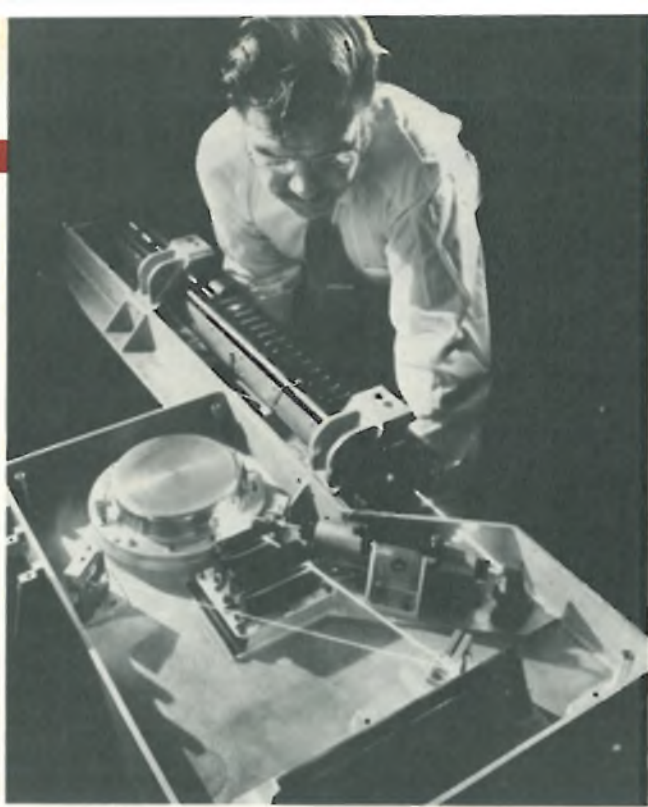
Laser writer. IBM's new 13,360-line-per-minute printer, model 3800, uses a low-power laser to form character images on a rotating drum, which picks up ink-like powder and transfers images to paper.
