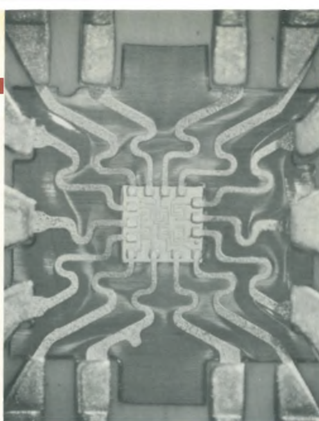
ICs on film. A familiar sight from now on will be the gang-bonded IC chip, like the RCA unit shown here on a frame of 9-mm film.
