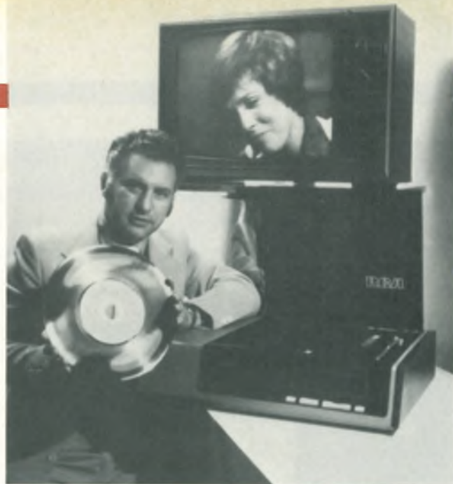
Video-disk entry. One video-disk system due on the market by the end of 1976 is this RCA capacitance-based player. It will compete against an optical system, due about the same time from MCA/Philips, and Teldec's already available mechanical system.
