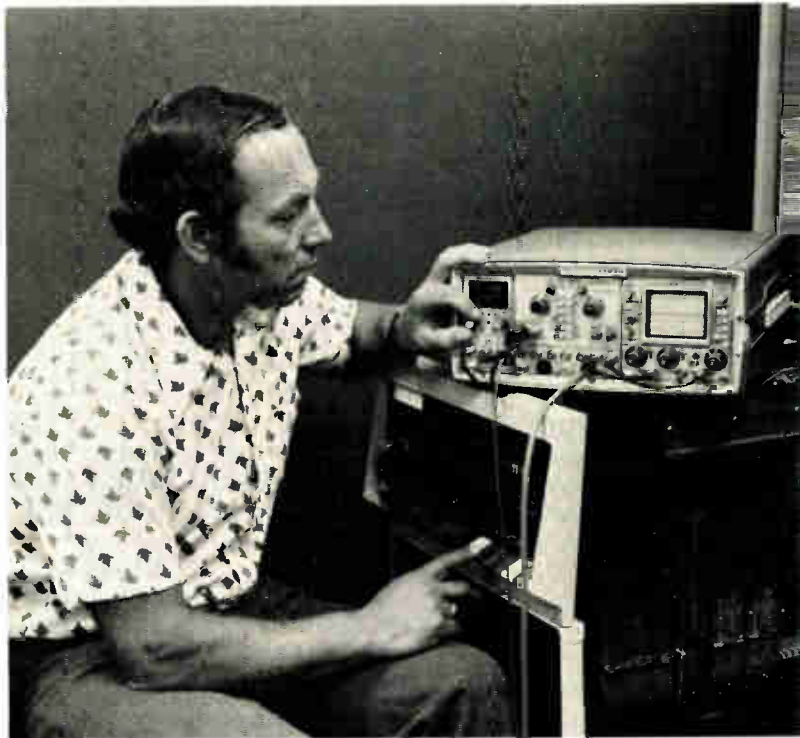
3. Viewing data. The latest oscilloscopes offer features aimed at digital testing in the lab or for field service. HP's model 1740A, for example, has a bandwidth of 100 MHz and an optional push button to alternate logic-state with time-domain displays.
