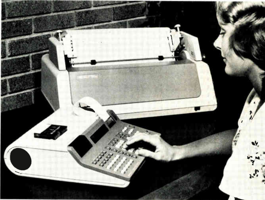
Micro control. Desktop calculator in foreground uses M6800 microprocessor from Motorola. But for its new page printer, Hewlett-Packard designed its own microprocessor.
