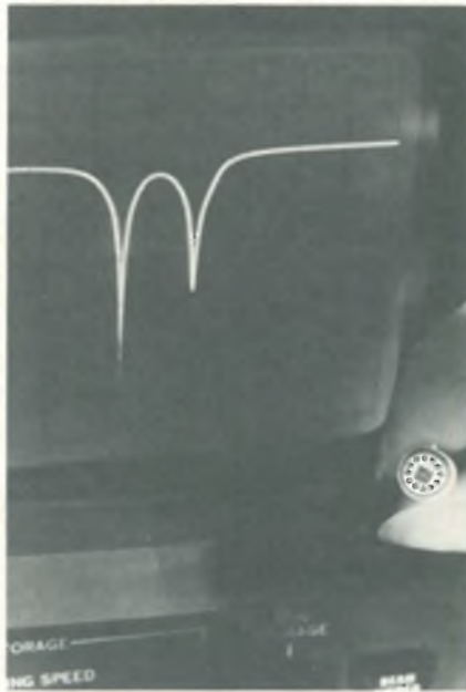
Filter chip. Gyrator circuits on integrated-circuit chip provide sharply tuned filtering (shown on the display) for color-TV sets.
