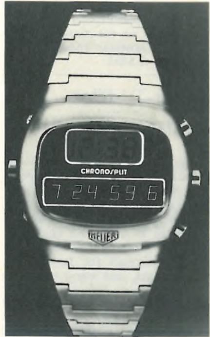
Double time. Combination watch and stopwatch from Heuer Time & Electronics and Integrated Display Systems has both liquid-crystal and light-emitting-diode displays.
