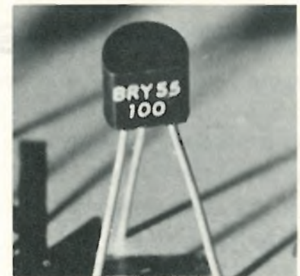
BRY 55 S planar thyristor in plastic package has a recovery time of less than 6 \mu s. Intended for switching power supplies and similar applications, the device has a voltage rating of 22 V and a current rise rating of 100 A/ \mu s. Sescosem, 50 rue J.P. Timbaud, 92400 Courbevoie, France [450]
