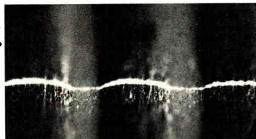
Checking the thickness of a fired print.
