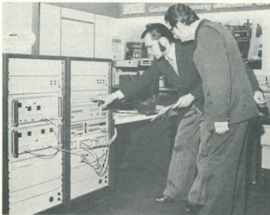
Testing. At Leipzig fair, Robotron 4200 computer controls station for testing and measuring parameters of components on pc boards.
