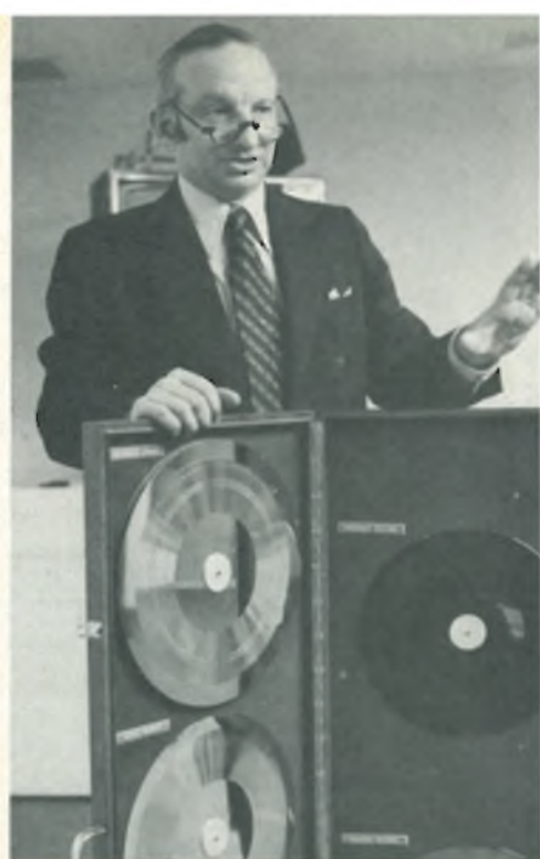
RCA's entry. Richard W. Sonnenfeldt, RCA staff vice president, introduces his company's video-disk system. Unlike Philips/MCA's, it uses capacitance-needle playback.
