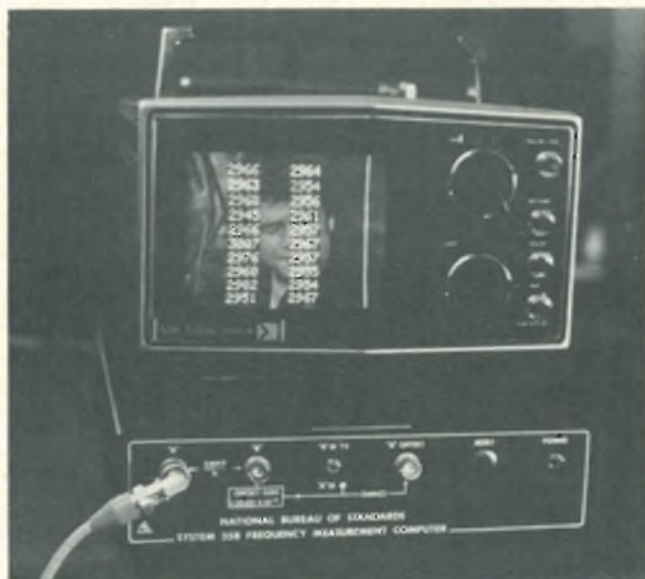
9. Computer. Frequency offsets and averages of 10 offset readings can be computed. The values can be displayed, along with a phase cursor, on a television screen.
