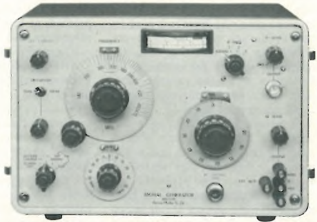
Signal Generator MG54B 335 to 470MHz
