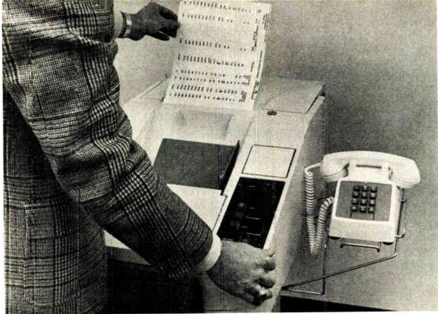
Plain fax. A helium-neon laser inside Xerox Corp.'s new two-minute facsimile machine creates images on plain paper, using the company's xerographic process.
