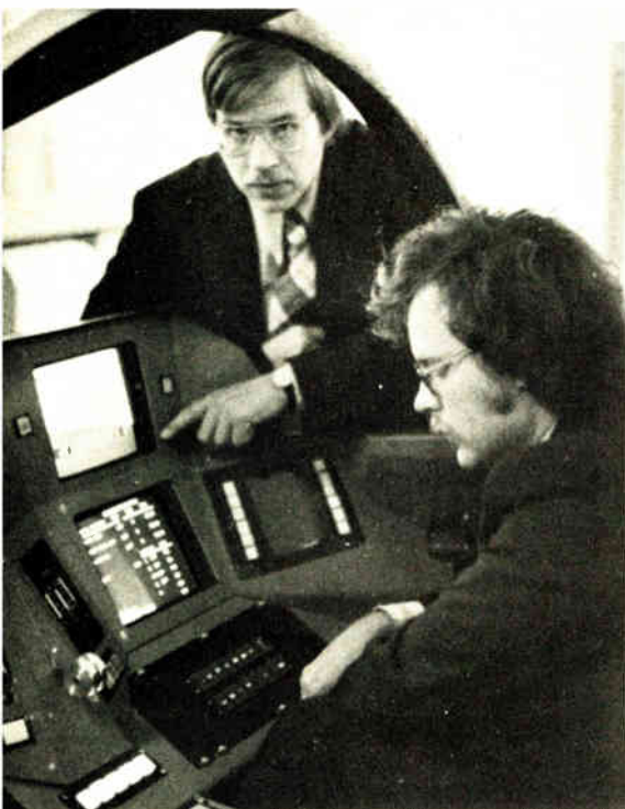
On the ground. This simulated cockpit is being used for R&D on the forthcoming avionics test bed for DAIS, a program for time-shared displays and controls.
