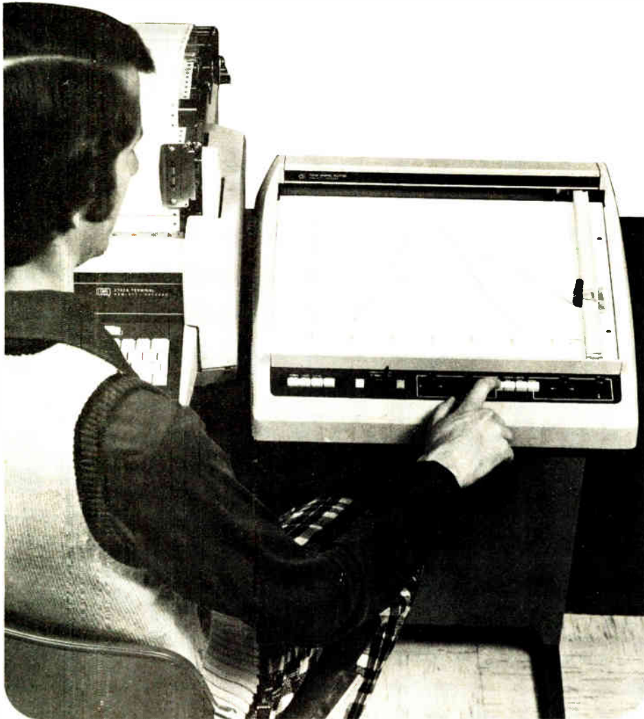
Fast digital X-Y plotter accepts bit-serial ASCII at 10 or 30 characters per second.
