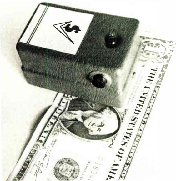
Recorder. Hand-held validator detects counterfeit U.S. currency by impressing magnetic signal on the printing inks.
